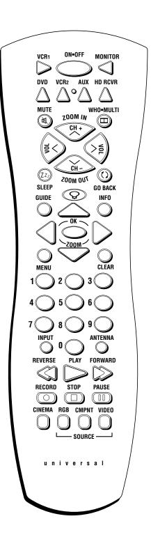
**ON•OFF** Toggles power on and off for the components that you have programmed. For example, if you are in VCR mode, turns VCR on and off.
